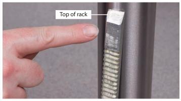
**4.** Fit the rise and fall rack into the square recess in the mounting body casting, ensure that it is engaged with the pinion, see figs 6 and lower the combined mechanism over the column (1). Allow it to slide down the column until the rise and fall rack is located in the cup chamfer in the top of the mounting flange, see figs 7. Replace the cup chamfered retaining
