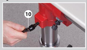
**3.** Locate another lift and shift handle (10) and screw it into the threaded hole for the Horizontal clamp assembly, see fig 22.
