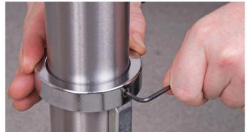
5. Locate and fit the crank handle (9) to the shaft, ensuring that you tighten the grub screw onto the machined flat on the shaft, this will keep the worm gear in position, see figs 9-10.
