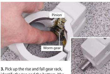
identify the top and the bottom, (the rack gearing is cut asymmetrically, with
