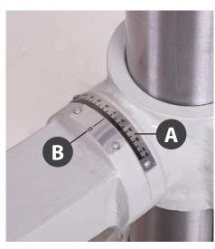
Table tilt scale (A) Table tilt pointer (B)
