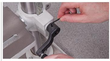
6. Check that the bracket can be driven up and down the column and can swivel around the pillar. Locate the lift and shift clamping handle (10) and screw it into the threaded hole to the rear of the mounting bracket arm (2) and tighten, see fig 11. Check it has 'pinched' up on the column and the bracket is immobile; both in its up and down travel and swivel movement.
