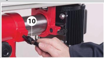
**4.** Open the pulley cover and check to see if the belt has been tensioned. If not, loosen the two motor yoke locks and push the motor back to tension the belt, see fig 23-24-25. For the floor standing pillar drill head, move the tensioning lever back then re-tighten the motor yoke locks to lock the motor in place, see fig 25-26.
