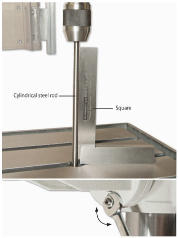
1. The cust iron table can be tilted 45° degrees in both plains, to tilt the table you will need to first remove the tables 90° locking pin. To remove the locking pin use a 10mm spanner, turn the nut clockwise to draw the pin out. Remove the pin and place safely aside, see fig 48-49. Loosen the tilt clamping bolt and tilt the table to the desired angle then retighten the bolt.
