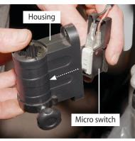
**6.** Line up the two holes in the micro switch unit with the threaded holes to the end of the angled bracket (6). **Make sure to introduce the micro switch cable into the cutout slot in the mounting bracket (6).** Secure the micro switch with two M5 Phillips screws (18), see fig 31.
