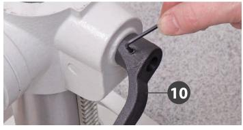
6. Check that the mounting bracket can be driven up and down the column and can swivel around the pillar. Locate the lift and shift handle (8) and screw it into the threaded hole to the rear of the mounting bracket arm and tighten, see fig 12. DO NOT OVERTIGHTEN as the cast iron arm could break. Check it has 'pinched' up on the column and the bracket is immobile; both in its up and down travel and swivel movement.
