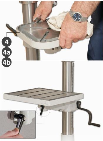
7. Screw in the remaining lift and shift handle (8) into the threaded hole to the end of the mounting arm. **DO NOT OVERTIGHTEN** as **the cast iron arm could break**. Lower the drill table (4,4a,4b) spigot into the machined hole to the front of the mounting arm and tighten the handle until it has 'pinched' up on the drill table's spigot and the table is immobile, see fig 13-14-15.
