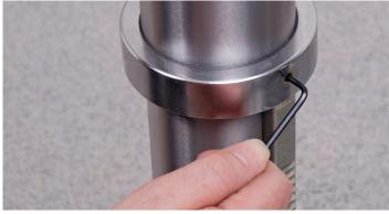
**5.** Locate and fit the crank handle (10) to the shaft, ensuring that you tighten the grub screw onto the machined flat on the shaft, this will keep the worm gear in position, see fig 10-11.
