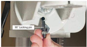
2. To set the table back to 90° degrees, loosen the clamping bolt, position the table back in the horizontal plain and insert the locking pin into the machined hole in the support arm. Adjust the nut so it protects the end of the threaded pin and using a high faced mallet tap the locking pin into place.
