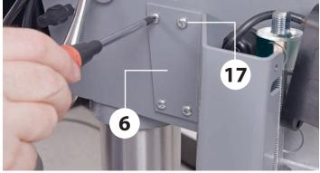
**5.** Insert the micro switch cable into the machined cutout slot in the mounting bracket (6). Press the switch assembly into the rear of the micro switch housing as shown, see fig 30.
