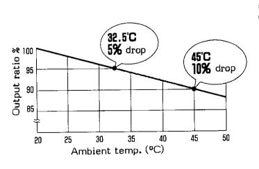
The engine's rated output is designed to have 100% output at 20°C. Take the effects of engine site and the temperature into consideration.
