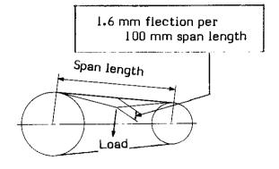
Measure the load with the spring scale
