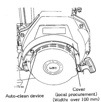
Installation of an "Auto-clean device" (optional part) to the cooling air inlet is recommended.
