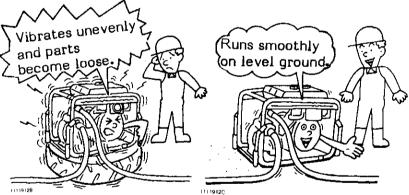
o Do not install the machine on a tire
