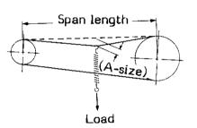
Flection load for proper belt tension, and the corresponding shaft load
