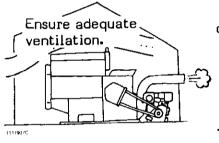
When using the engine indoors, be sure to provide adequate ventilation.
