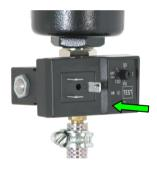
9. Place the connector gasket on the connector, plug the connector on the timer as illustrated below and tighten the screw (max. torque 1Nm) and make sure both gaskets are secured properly to ensure IP65 rating.
