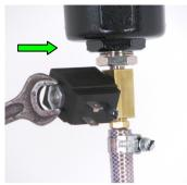
The coil can be rotated 360° around the valve, you can align the coil as desired.
