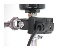
6. Unscrew the valve shaft using a 13 mm wrench.
