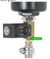
Make sure there is no debris between the gasket and the coil.
