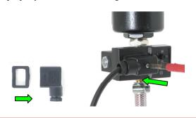
6. Place the flat gasket over the coil connection pins.
